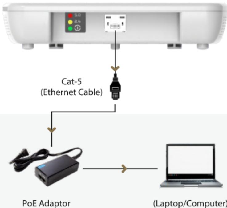
3. Open the web browser and enter the Access Point static IP address in the address bar: 192.168.1.1
